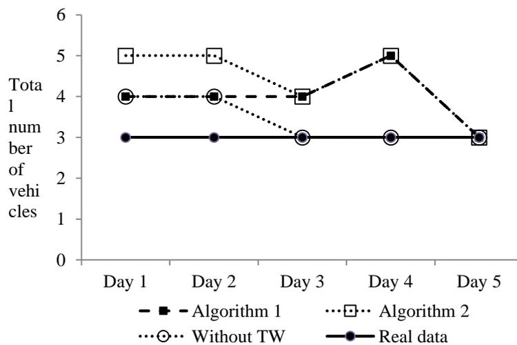
Also the use or possible adjustment of time windows influences the results regarding the total number of vehicles obtained by the savings algorithm. Algorithm 1 seems to be more promising than algorithm 2, since it computes in none of ten cases a higher number of vehicles than algorithm 2 does. At the same time it delivers a lower number of vehicles than algorithm 2 does for three cases.
