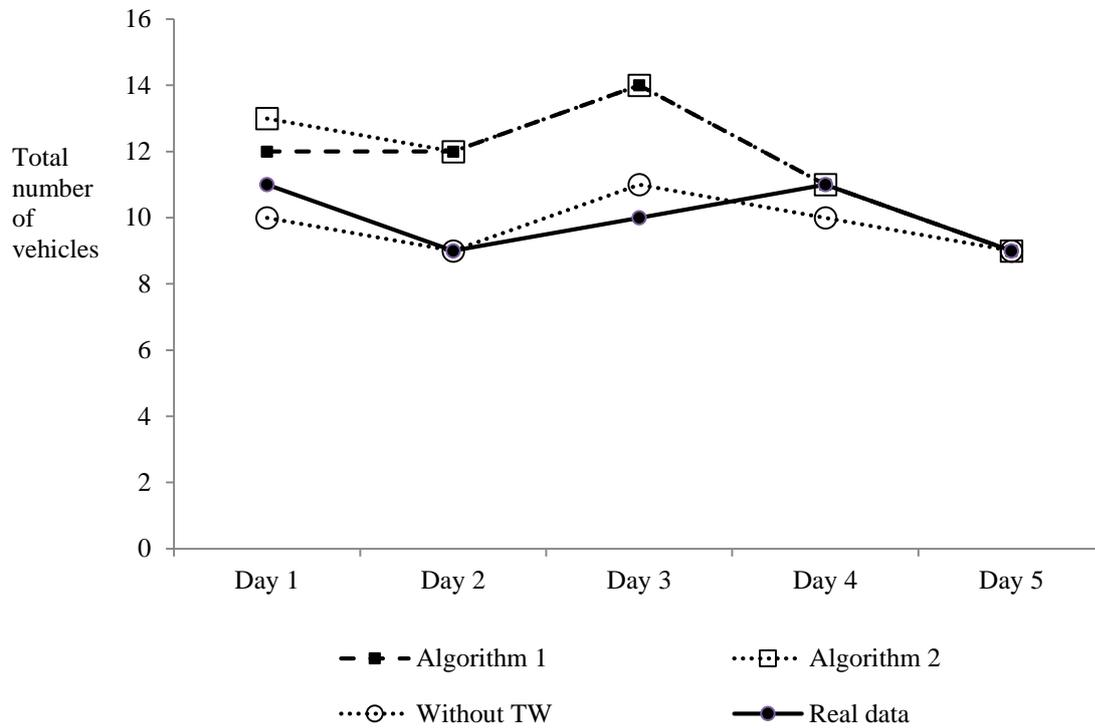
The differences between the numbers of used vehicles for organic waste are presented in figure 6. The number of vehicles for the configuration without time windows again equals the number of clusters. Algorithm 2 delivers weaker results for the days 1 and 2, since the solution contains one vehicle more. The result of the cluster algorithm mainly influences the number of vehicles necessary to serve all demands.
